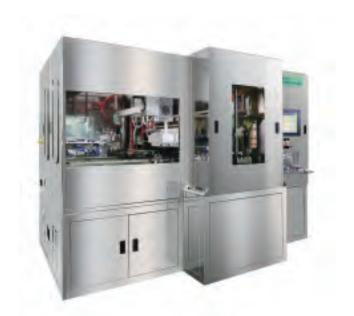
The MW 600C is a plasma cleaning and de-smearing system specifically designed for panel level product and PCB after the drilling process. The system is comprised of three stations, with loaders and unloaders on both sides, and a plasma chamber with lifter in the center. The main plasma source for the MW 600C is microwave power.
